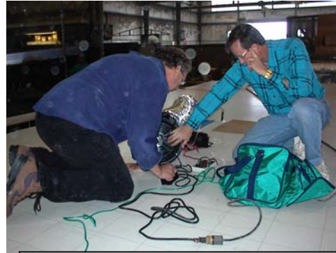
Duct tightness testing in the plant. This home section has no air handler unit so testing equipment is connected to a supply opening.
