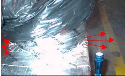
Smoke is seen leaking under the collar flange.
