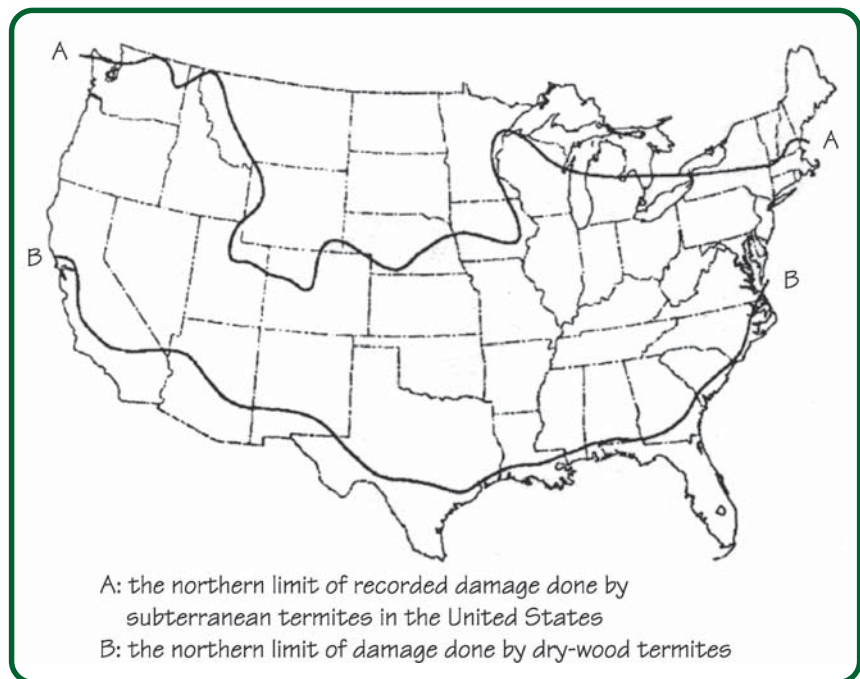
Figure 6.2 - Extent of Recorded Termite Damage
