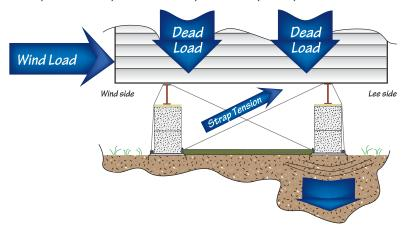
Figure 4.35 The dynamics of the Vector system.
