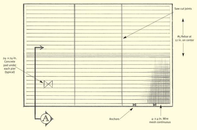
Figure 3.52 The slab design calls for anchors embedded in the concrete and saw-cut joints for expansion.
