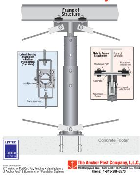
Figure 4.29 Storm Anchor details.
