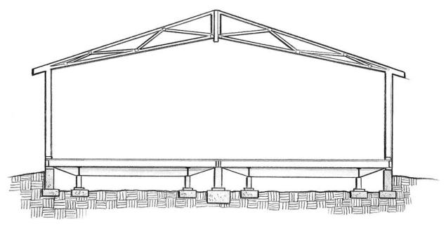
Figure 3.8 Crawl space foundation with full perimeter support, in low-profile configuration.
