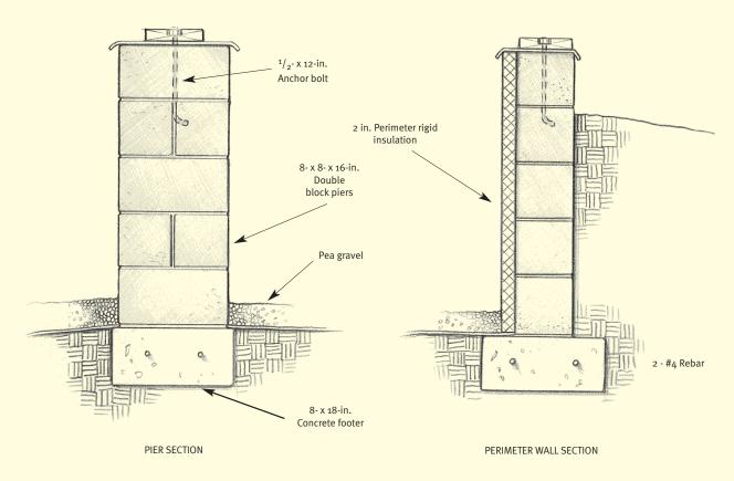
Figure 3.37 Cross section view showing perimeter and mating line supports for this recessed foundation system.
