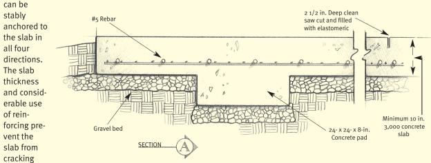
**Figure 3.53** The generously proportioned slab is thicker at loading points.
