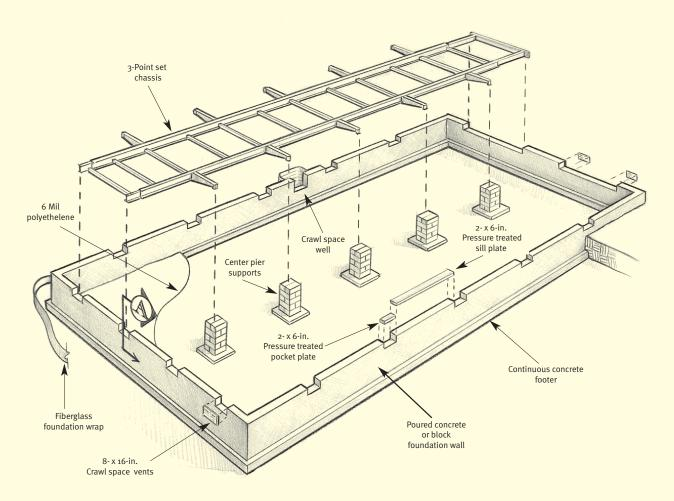
Figure 3.42 Isometric diagram showing cutouts in the exterior foundation wall to accommodate the loadcarrying outriggers.
