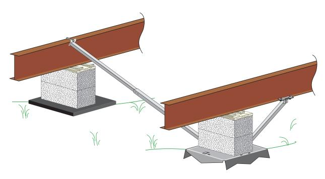
Figure 4.38 Xi Wind Zone 1 with concrete pier lateral and longitudinal systems.
