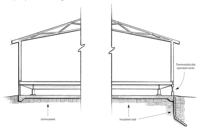
**Figure 3.45** A slab supports the home on top of the earth. The slab is uninsulated or insulated, depending on the local conditions and goals of the designer.
