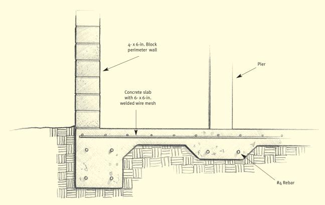
Figure 3.54 Asset Development also uses a thinner slab providing a more economical use of poured concrete.
