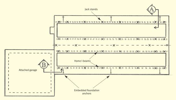
**Figure 3.39** Plan view of the foundation system showing points of support for the chassis.
