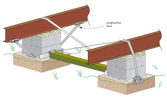
Figure 4.33 Vector Dynamic's lateral and longitudinal components for poured concrete.
