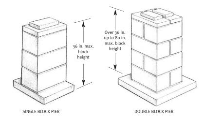
**Figure 3.3.** Common configuration of concrete block piers.
