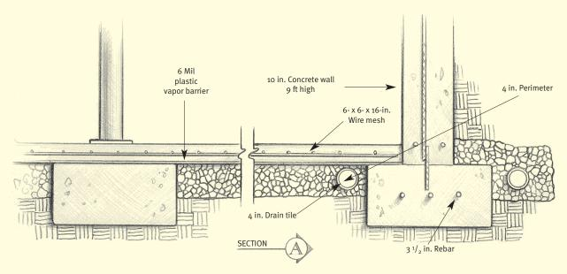
Figure 3.71 Cross section of basement showing structural reinforcing and techniques to keep the basement dry.
