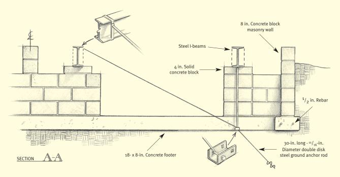
**Figure 3.35** Cross section of foundation system showing earth berming and connection to ground anchors.
