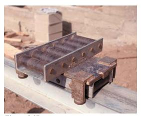
**Figure 3.67** A typical roller system for conveying a home onto its foundation.
