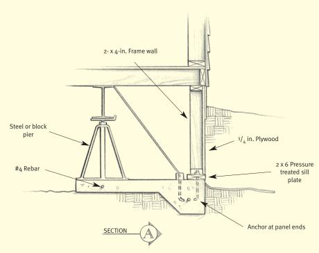
**Figure 3.40** The weight of the home is transferred to the ground by jack stands and stablilized by anchors.
