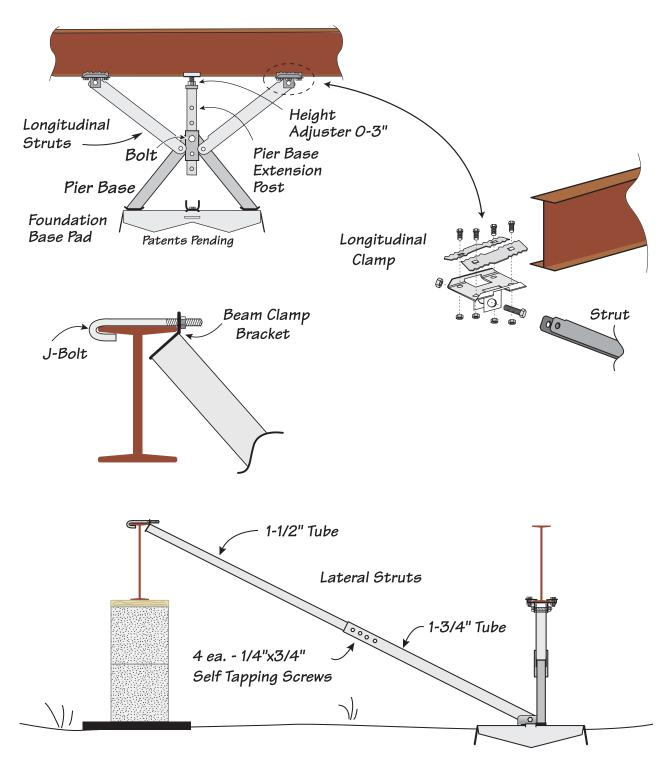
Figure 4.41 All components hot galvanized coated.
