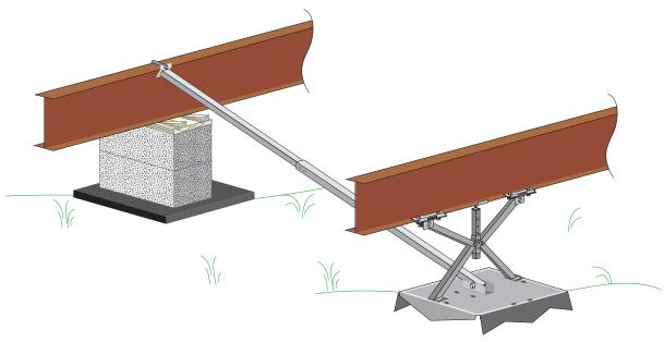
**Figure 4.39** Xi Wind Zone 1, 2 or 3 with steel Xi pier lateral and longitudinal.
