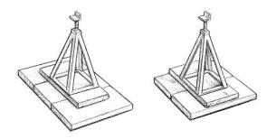
Figure 3.4. Triple and double pad footings.
