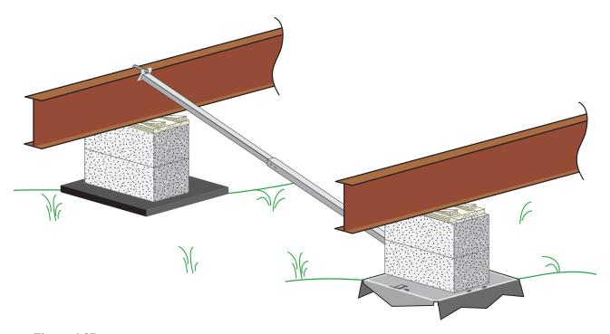
**Figure 4.37** Wind Zone 1 with concrete pier lateral system.
