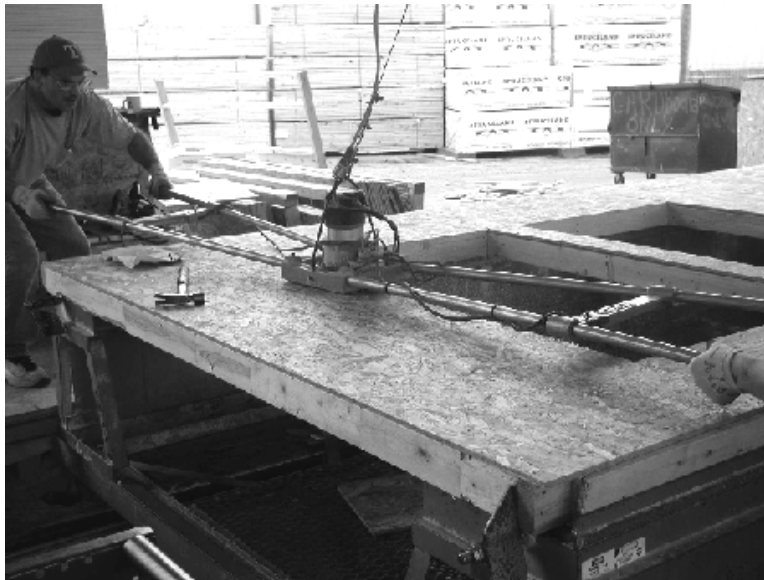
Figure 19 Machining of Panel Openings
