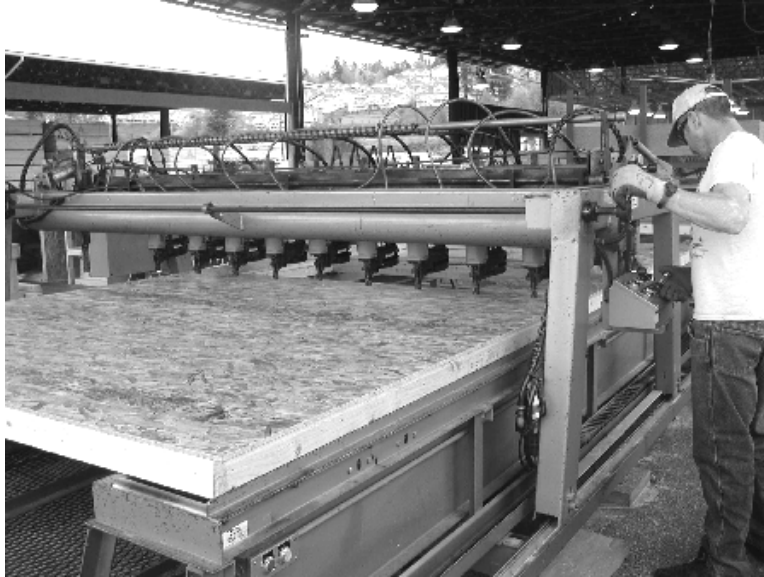
Figure 20 Multiple Nail Gun Rack for Attaching Sheathing Panels
