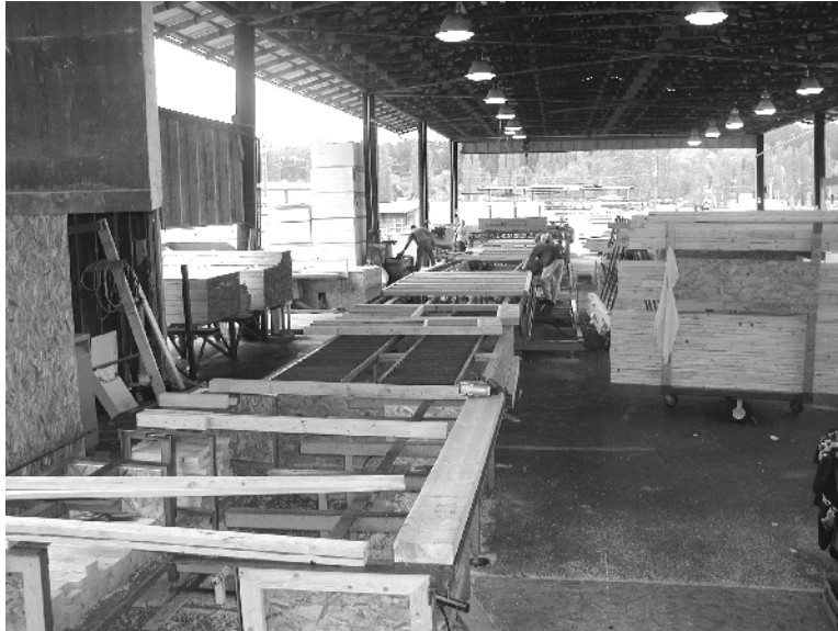
Figure 16 Wall Panel Production Line
