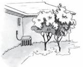
Shading an outdoor compressor can improve energy efficiency
