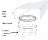
The crossover duct connection must be tightly sealed
