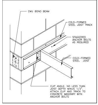
Figure 2-7: Cold-Formed Steel Floor Ledger Connection
