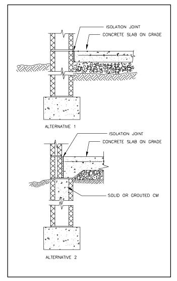
Figure 1-1a: Foundation Stem Wall and Slab on Grade
