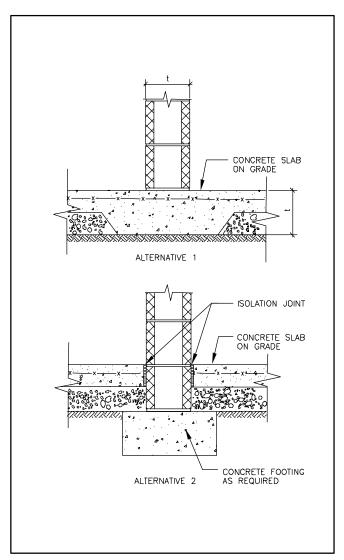
Figure 1-3: Interior Bearing-Wall Foundation
