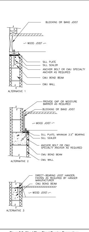
Figure 2-2: Wood Floor Direct-Bearing Connections
