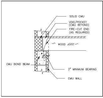
Figure 2-1: Wood Floor Pocket Connection
