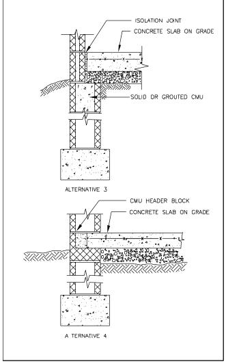
Figure 1-1b: Foundation Stem Wall and Slab on Grade
