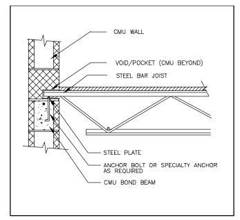
Figure 2-8: Steel Joist Floor Direct-Bearing Connection
