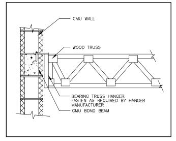
Figure 2-4: Wood Truss Floor Direct-Bearing Connection
