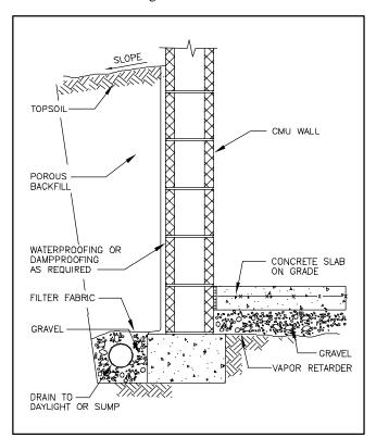
Figure 1-6: Moisture and Water Control Measures
