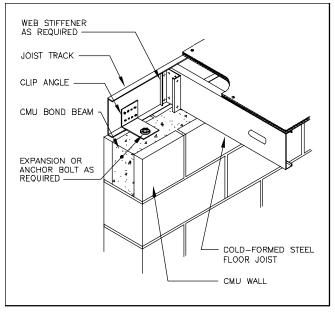
Figure 2-6: Cold-Formed Steel Floor Direct-Bearing Connection
