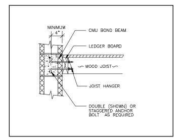
Figure 2-3: Wood Floor Ledger Connection
