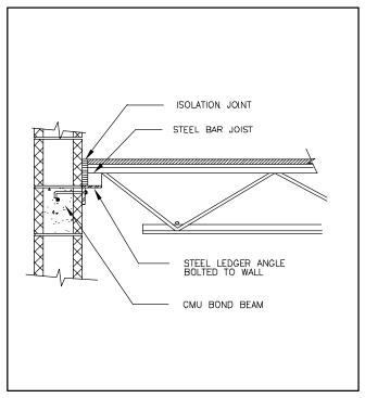
Figure 2-9: Steel Joist Floor Ledger Connection
