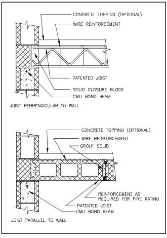
Figure 2-10: Block Joist<sup>a</sup> Floor System
