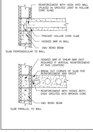
Figure 2-11: Precast Concrete Floor Direct-Bearing Connection
