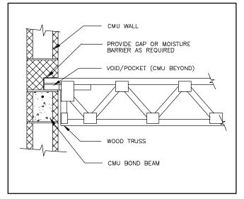
Figure 2-5: Wood Truss Floor Pocket Connection
