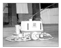
Figure 2.3: Concrete finishing robot
