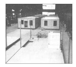
**Figure 2.2:** Modular housing on the factory floor *Source: HUD*
