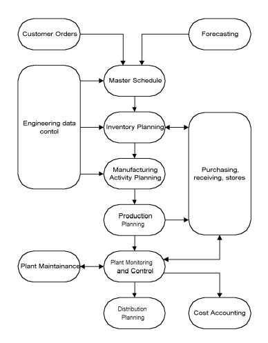
**Figure 2.6:** Typical MRP II system and its modules. *Source:* Meredith and Shafer 1999, p. 276.
