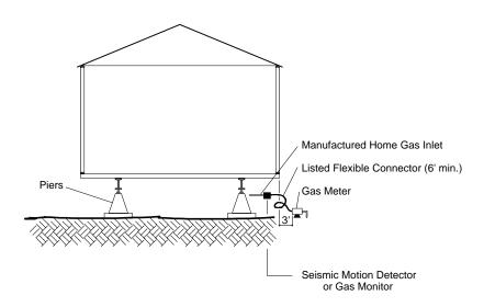
Lot size and offset requirements may not always allow three feet between the meter and the home. Further, the flexible connector may be damaged by lawn mowers or children playing around the home and must, therefore, be protected from damage.
