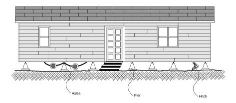
Detachable hitches may be removed and stored under the front of the home directly under the chassis beams. The axles and hitch will prevent the home from falling completely to the ground in the event of an earthquake.
