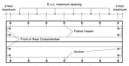
Anchor Minimum Load Capacity 4725 lbs.
