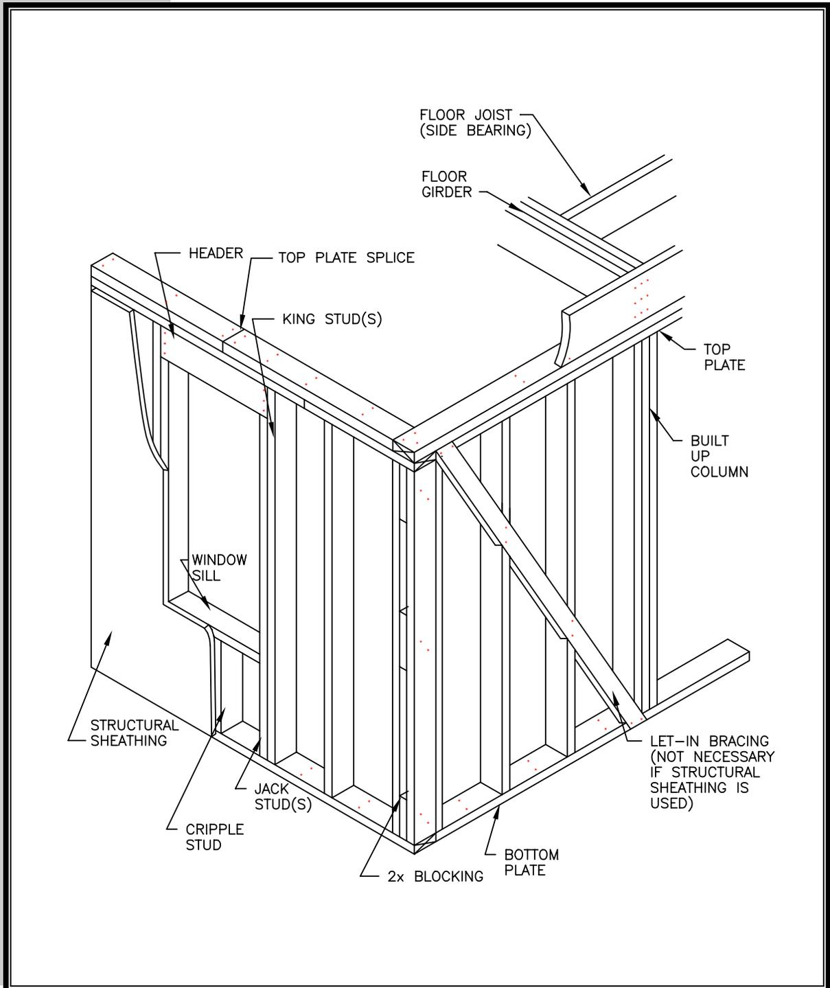
Structural wall sheathing, such as plywood or oriented strand board, distributes lateral loads to the wall framing and provides lateral support to both the wall studs (i.e., buckling resistance) and the entire building (i.e., racking resistance). Interior wall finishes also provide significant support to the wall studs and the structure. In low-wind and low-hazard seismic areas, metal ‘T’ braces or wood let-in braces may be used in place of wall sheathing to provide resistance to
