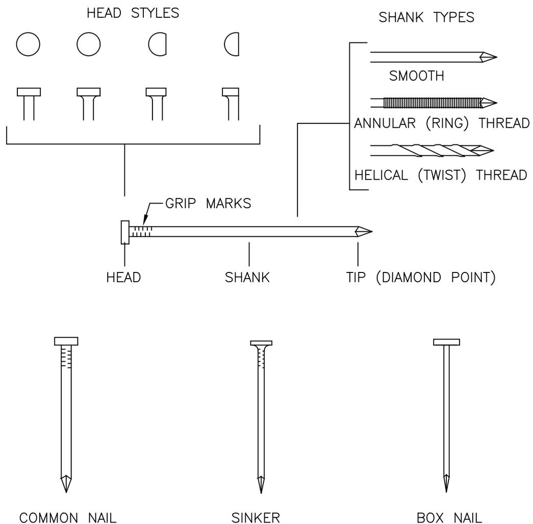
The following are the most common nail types used in residential wood construction.
