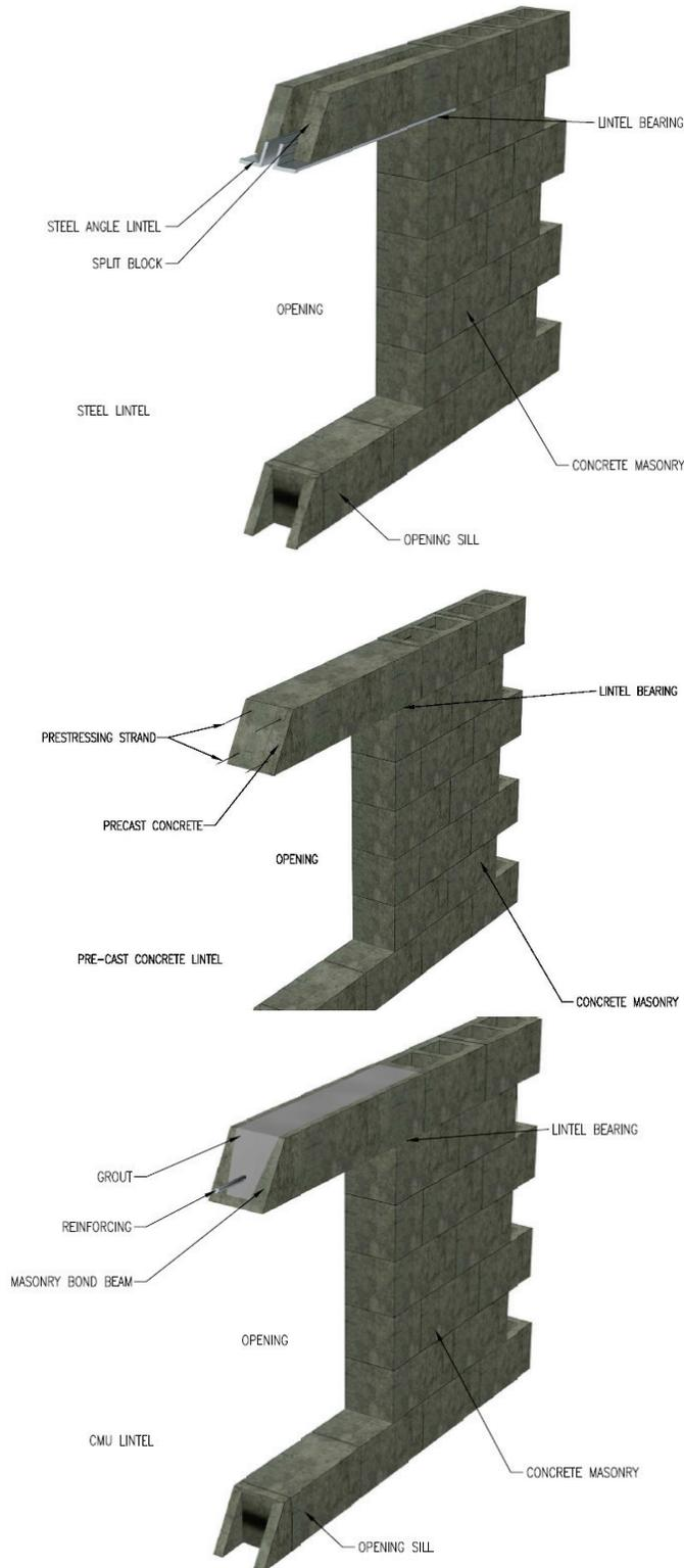
Many prescriptive design tables are available for lintel design. For more information on lintels, arches, and their design, refer to the National Concrete Masonry Association's (NCMA's) TEK Notes. Information on lintels and arches also can be found in *Masonry Design and Detailing* (Beall, 2012).
