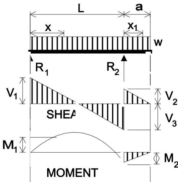
$$R_1 = V_1 = \frac{w}{2L} (L^2 - a^2)$$
