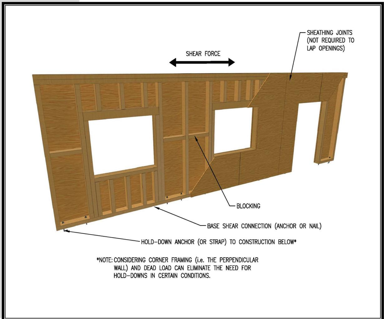
The PSW design method requires the least amount of special construction detailing and analysis among the current shear wall design methods. It has been validated in several recent studies in the United States but dates back more than 20 years to research first conducted in Japan (Dolan and Heine, 1997a, 1997b; Dolan and Johnson, 1996a, 1996b; NAHB, 1997, 1998, 1999; Ni et al., 1999;
