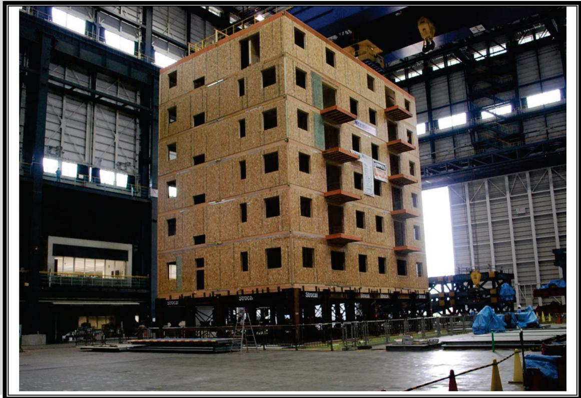
The Insurance Institute for Business and Home Safety has built a full-scale wind tunnel to support the research done for their insurance constituency. To date, the institute has conducted wind testing on several full-scale houses and performed important component testing of siding materials and rooftop equipment. Their full-scale facility also has tested products and systems for wildfire, hail, and wind-driven rain.
