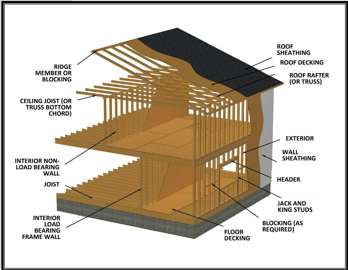
Each system can be complex to design as a whole; therefore, simple analysis usually focuses on the individual elements (subassemblies) that constitute the system. In some cases, “system effects” may be considered in simplified form and applied to the design of certain elements that constitute specifically defined systems. Structural elements that make up a residential structural system include—
