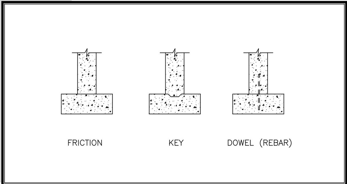
***Friction Used To Provide Shear Transfer***
