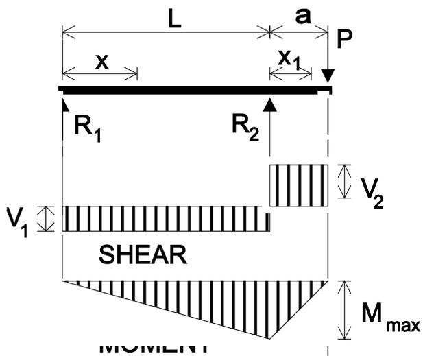
$$R_1 = V_1 = \frac{Pa}{L}$$
