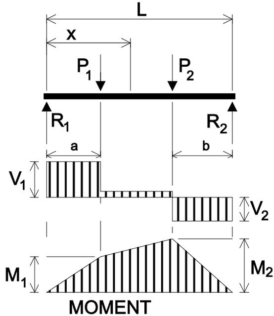
$$R_1 = V_1 = \frac{P_1(L - a) + P_2 b}{L}$$
