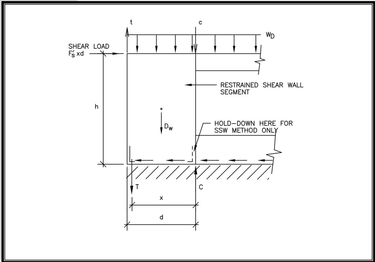
For a more simplified analysis of overturning forces, the effect of dead load may be neglected (the normal case in practice) and the chord forces determined as follows, using the symbols defined as before.
