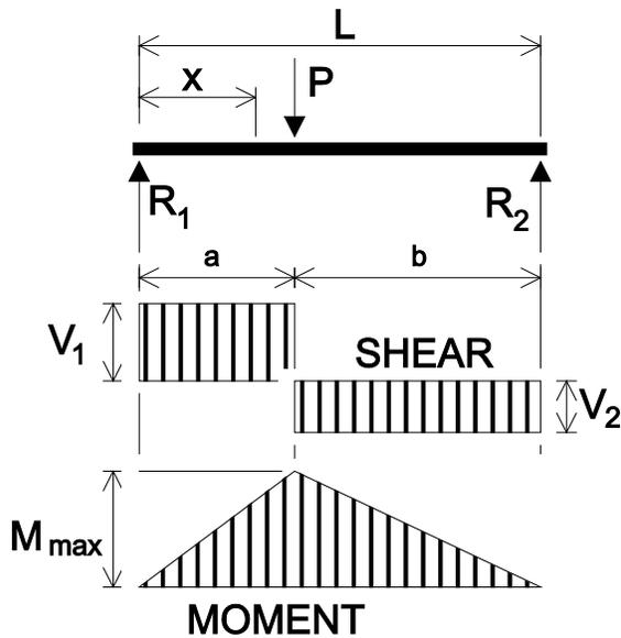
$$R_1 = V_1 \text{ (max when } a < b) = \frac{Pb}{L}$$
