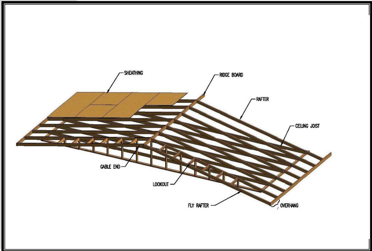
Roof trusses are pre-engineered components. They are fabricated from 2-inch thick dimension lumber connected with metal truss plates. They are generally more efficient than stick framing and usually are designed to span from exterior wall to exterior wall with no intermediate support. Complex portions of roof systems, however, often use rafter-framing techniques.
