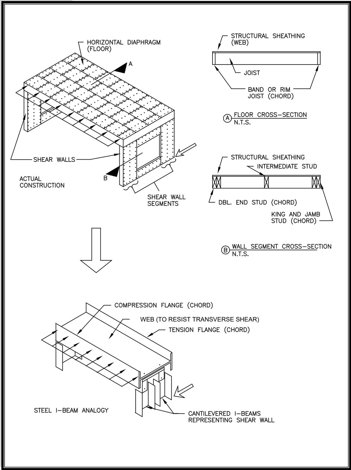
**FIGURE 6.4** *Shear Wall Collector and Composite Failure Plane*
