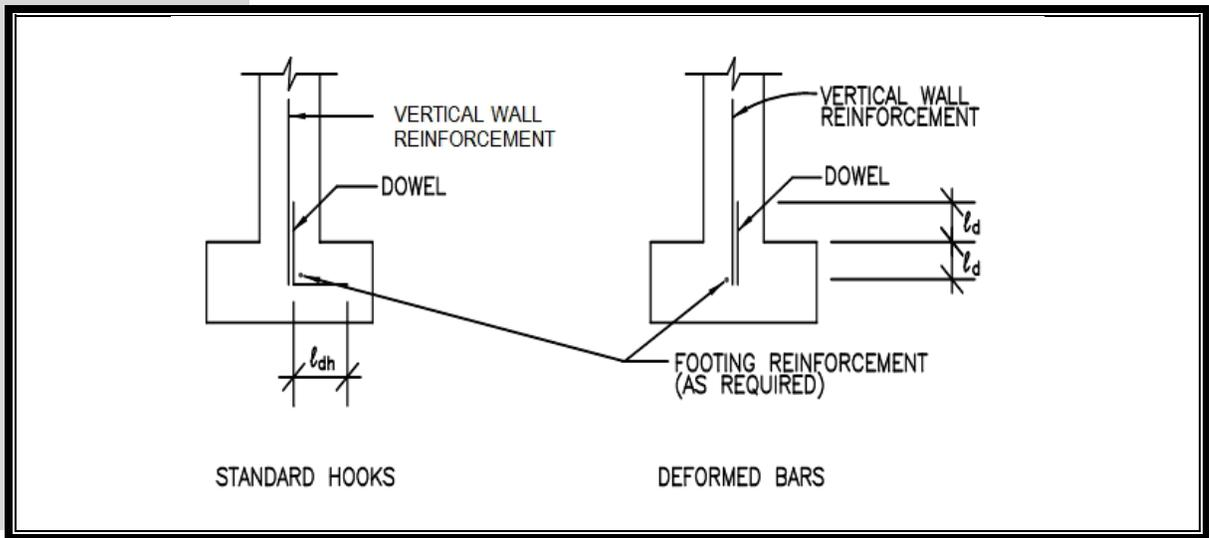
The minimum embedment length is a limit specified in ACI-318 that is not necessarily compatible with residential construction conditions and practice; therefore, this guide suggests a minimum embedment length of 6 to 8 inches for
