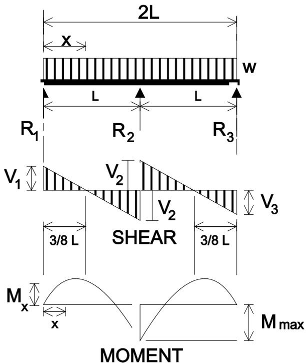
$$R_1 = V_1 = R_3 = V_3 = \frac{3wL}{8}$$
