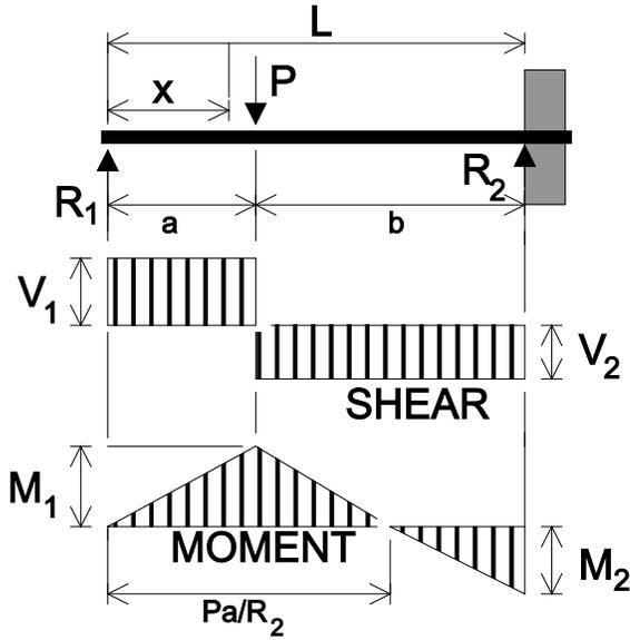
$$R_1 = V_1 = \frac{Pb^2}{2L^3} (a + 2L)$$
