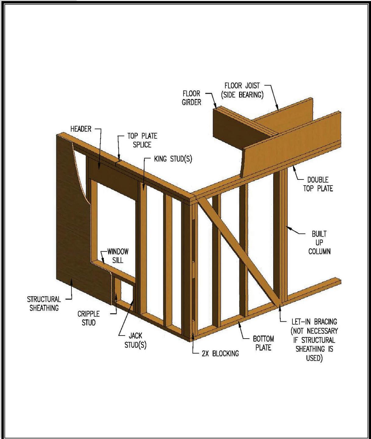
Structural wall sheathing, such as plywood or OSB, distributes lateral loads to the wall framing and provides lateral support to both the wall studs (that is, buckling resistance) and the entire building (that is, racking resistance). Interior
