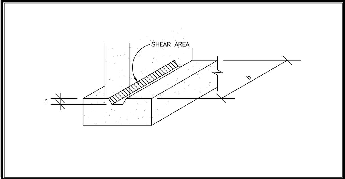
***Dowels Used To Provide Adequate Shear Transfer***
