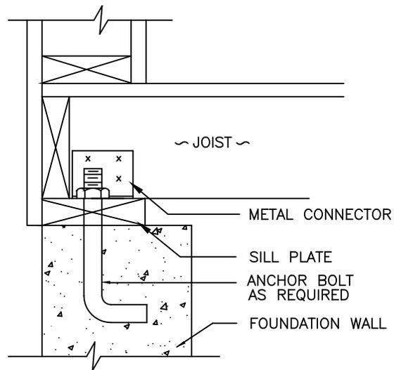
**Conclusion** This example demonstrates an analytic method of determining foundation lateral loads and the required connections to support the top of the foundation wall through a wood sill plate and floor construction. It also demonstrates the discrepancy between calculated connection requirements and conventional construction experience that may be negotiated by permissible designer judgment and use of conventional residential construction requirements.
