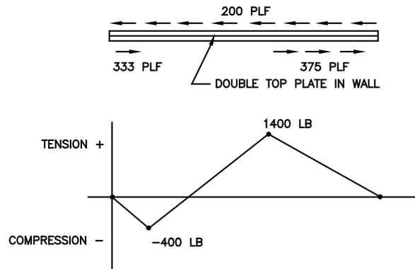
The first point at the interior end of the left shear wall segment is determined as follows—
