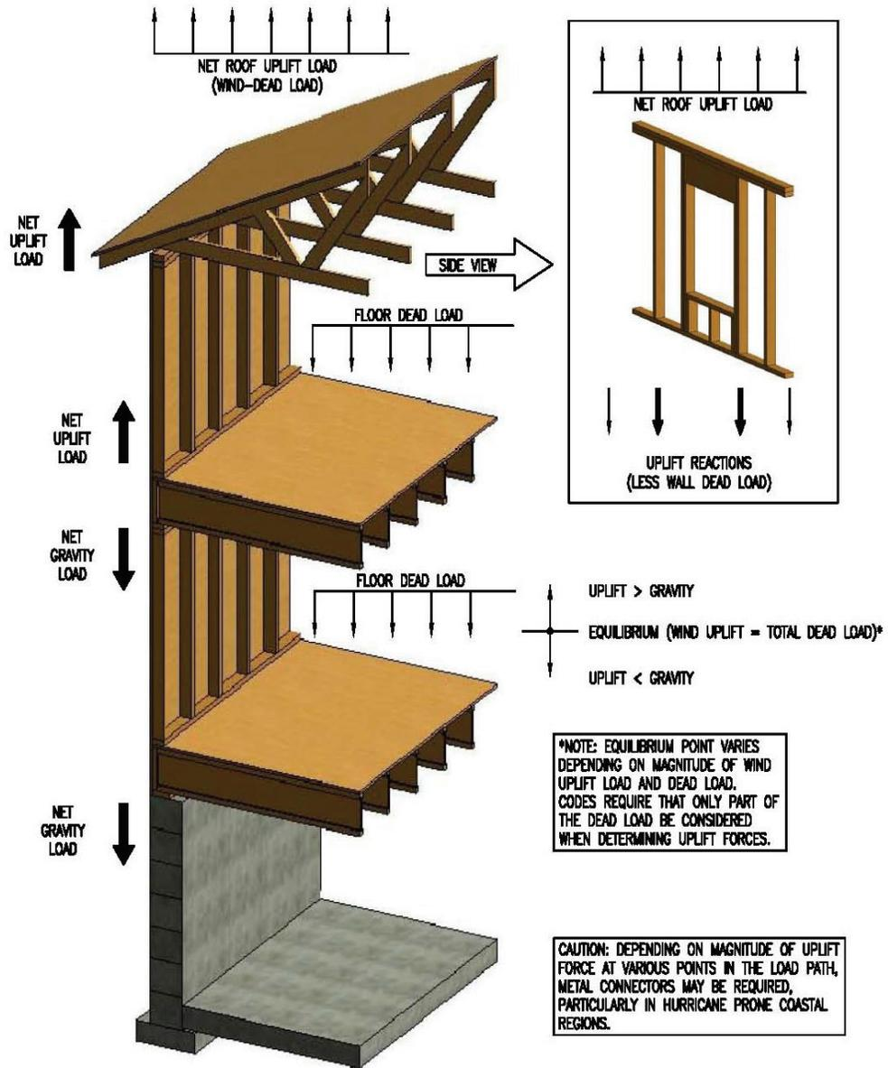
In a typical two-story home, the load path for gravity loads and wind uplift involves the following structural elements—
