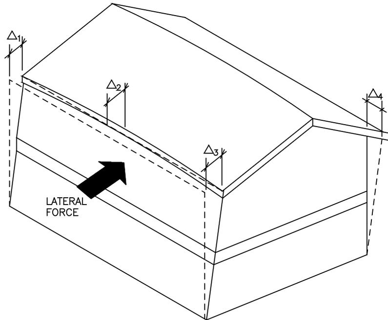
NOTE: IF STIFFNESS OR LOAD IS NONSYMMETRICAL, BUILDING ROTATION OCCURS ( $\Delta_1 \neq \Delta_3$ ) AND LOADS ARE DISTRIBUTED BY TORSION ( $\Delta_4 \neq 0$ ) AS WELL AS BY DIRECT SHEAR IN THE DIRECTION OF THE LATERAL FORCE. THIS CONDITION VARIES BUT IS A REALITY FOR MOST DESIGNS.  $\Delta_2$  IS THE BENDING DEFORMATION OF THE HORIZONTAL DIAPHRAGM (I.E., ROOF).
