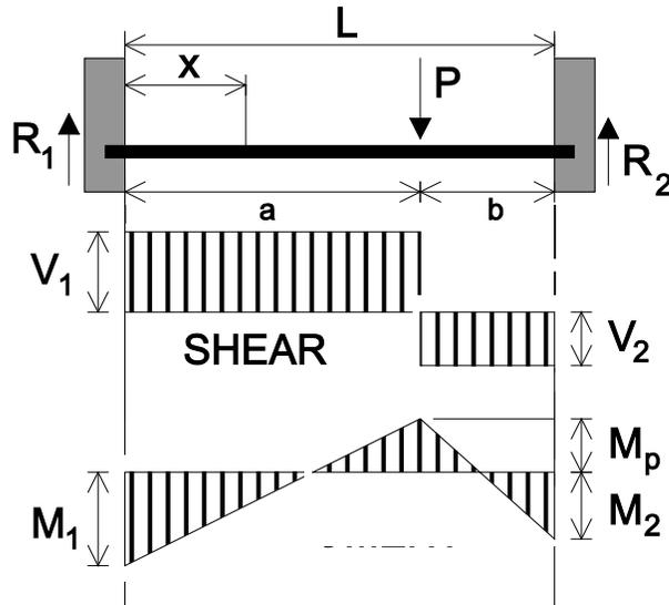
$$R_1 = V_1 \text{ (max. when } a < b) = \frac{Pb^2}{L^3} (3a + b)$$
