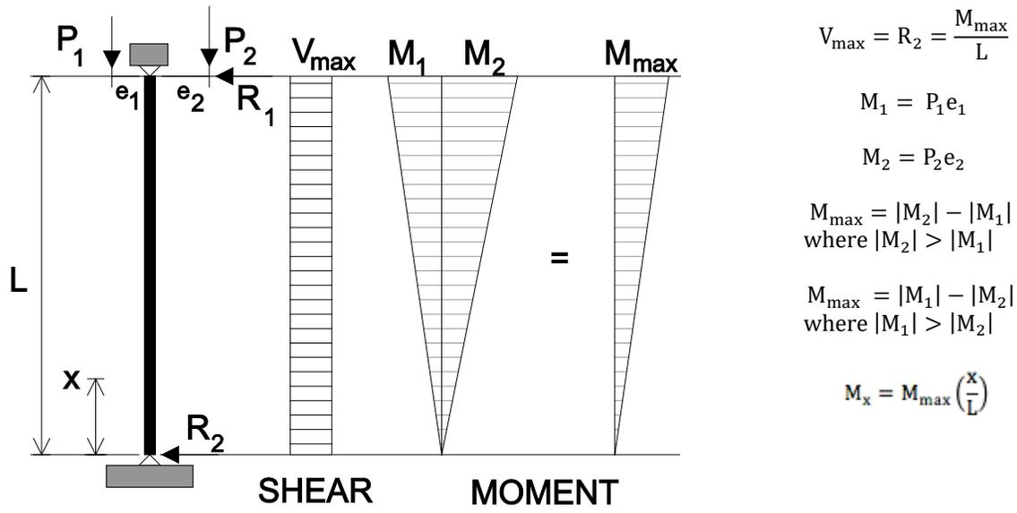
Figure A.2. Simple Beam (Wall or Column)—Eccentric Point Load
