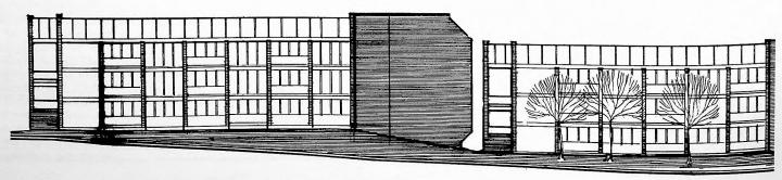
Roof for apartment structures may be precast panels, similar to the floor units, or steel roof decking may be used, with either covered by built-up roofing. Exterior finish may be a variety of materials, but the use of structural clay brick units is recommended for esthetic considerations and value in savings on maintenance. Balconies, with sand-blasted concrete railings are planned for all living units.
