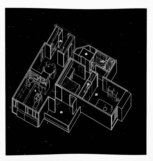
Terrazo-finished floor and painted gypsum board ceiling may be integral with the modules. Insulation against both heat and cold is afforded by the material of the "hard" module itself—lightweight concrete.
