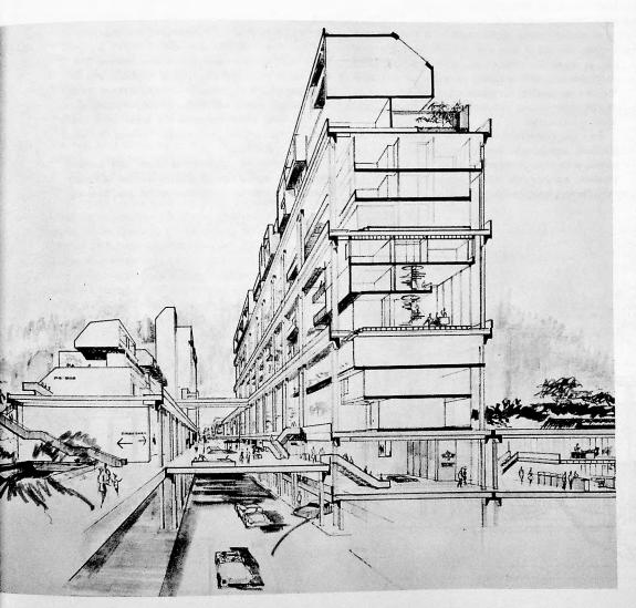
stair and slab elements added as required. House units placed on these decks or tiers are built around a core unit, 12 ft. x 15 ft. or 12 ft. x 20 ft. (depending on the size of the dwelling), which includes a steel stairway with a choice of various finishes; the heating unit, airconditioning ductwork, vertical utilities run, and the kitchen (with factory-assembled cabinetry, connections for choice of appliances, finish flooring and base, and raceways for electrical wiring and appliances).
