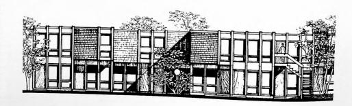
Onsite, the modules are set on conventional foundations and joined with others side-by-side, end-to-end or stacked two high. Where modules are to be joined, corresponding exterior and interior skins of the modules are omitted from the framework during plant assembly.
