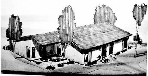
"Honeycombing" of the modules in building up dwelling units is expected to result in lower overall cost because approximately 100 percent more living space can be gained through use of the space enclosed between the modules, without any loss in overall structural strength of the low-rise project.
