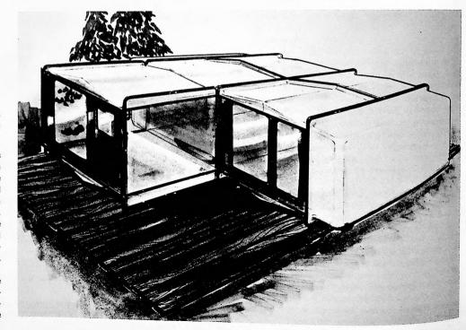
elements are produced by the open mold process; the sandwich consisting of a layer of fiberglass-reinforced polyester (FRP), a urethane foam core, and another layer of FRP.
