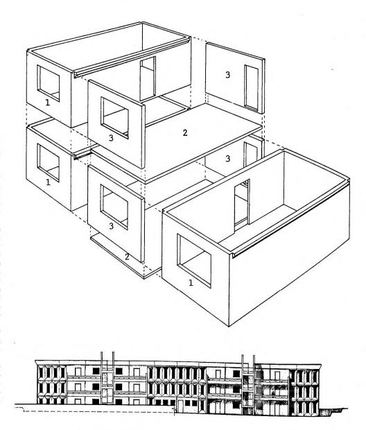
All piping can be incorporated in the units; kitchens and bathrooms are factory-fabricated for packaged field installation; other interior items can be prepared in the same way. Heating, cooling, and electrical subsystems are also included in the units, for easy connection with adjoining sections and only field connection to main supply lines. Heating may be supplied by gas or electricity.
