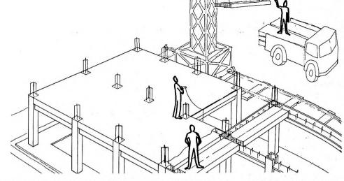
tity. Beams of the perimeter of the building have a slab high vertical edge or spandrel which serves as a form and becomes part of the completed slab. With slabs in place and completed, the cycle is repeated for the next floor.
