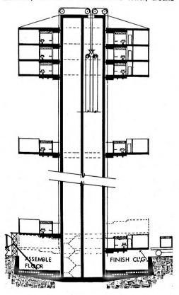
which are constructed at ground level, circular floor slabs, each slab being hoisted up the tower as completed. The floor slabs, structural entities in themselves, are supported by the central core structure from which they radiate.
