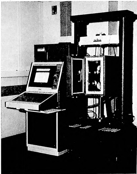
FIGURE 36 CONTROLLED HUMIDITY CHAMBER USED FOR TESTING STRENGTH OF ADHESIVE USED IN PANELS WITH FIBERGLASS REINFORCED POLYESTER SKINS
