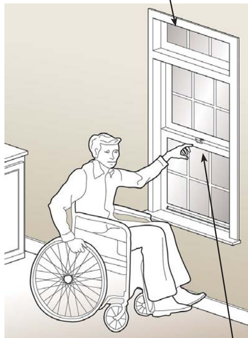
Resident opening a double hung window. Other types of windows such as horizontal sliding or awning types may be used
