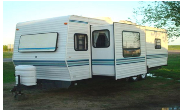
Travel trailer with “slide-out” provides additional interior area required for an accessible plan
